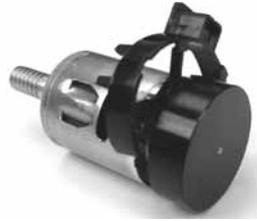
*Spread the Tach Reader bracket apart and slip between the flywheel and motor for engines equipped with Mabuchi or similar motors.*
