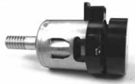
*Push the bracket all the way onto the top of the motor. The small tabs extending down will "lock" onto motor casing.*
