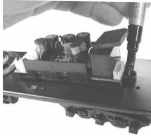
*Drill the appropriate mounting holes as determined from positioning the PS-2 board and other components*
