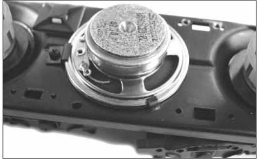
*Use the existing speaker location (if applicable) to mount the new speaker. Many diesel engines will use the fuel tank to house the speaker. Use the same mounting hardware for the original speaker.*
